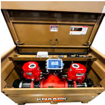
Chevron automated valve trial to manage fluid levels - project specific technology created for spill mitigation from Buffer to C-ring pumps
